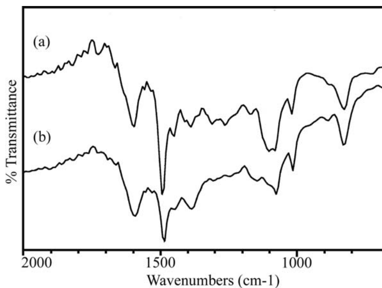
Figure 9. FT-IR spectra of (a) P4BAN before doping and (b) P4BAN after doping with iodine for 13 days at room temperature.
